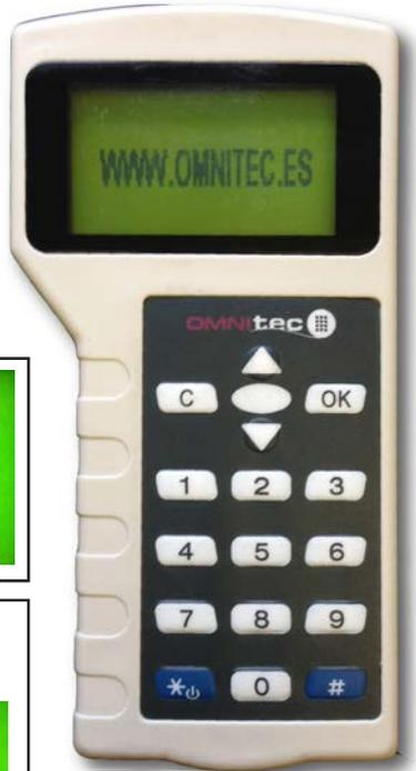
With the USB connected to the handheld programmer, switch on the unit. You can do this by pressing and holding the \* button at the bottom left. Once you see the ONMITEC welcome screen, press the OK button.
